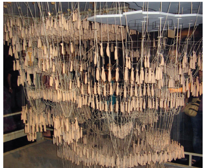
Gaudi's model using the hanging chain method to determine force distributions during structural design. The model is inverted.
